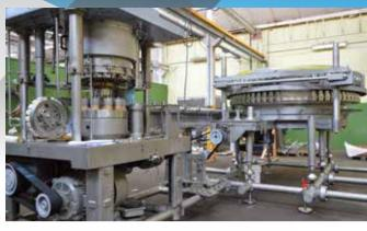
Complete machine rebuild of a 10-head X59 seamer synchronized with a high-capacity filler with 66 fill stations. Output 800 to 1200 cpm. Upgraded with full automatic lubrification and C.I.P. skid for dairy applications.
