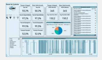
The main iOPS® dashboard contains high level key performance indicator statistics for measuring OEE, Availability, Productivity and more. Click on any of the information buttons on the main dashboard to drill down to detailed granular KPI data. All dashboards generate reports and filter by date ranges, with drill down by
