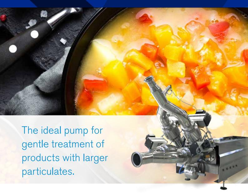
The Pumpideal<sup>™</sup> has been specifically developed to treat products with large particulates up to 80mm (~3.15") in size. Gentle product treatment is obtained at a maximum throughput of 10000 l/h (44 gpm) and an operating pressure of 15 bar (~218 psi).
