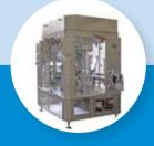
Seamer Places and seams the can end to the can
