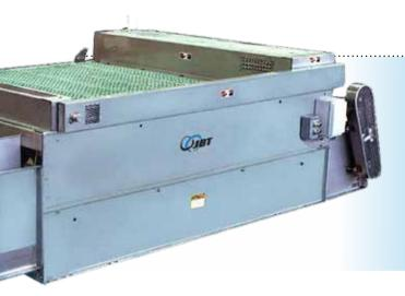
corrosion-resistant adjustment screws. This enables the module's movable frame, with its sizing rollers, to be raised or lowered easily. A calibrated scale readily permits direct reading of the size for which the module is set. The accuracy of this control, combined with precision fabrication of the modules, gives a sizing reliability unmatched by any other sizer.
