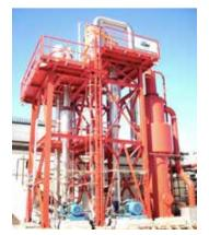
Compact Hot Break enzyme inactivator and TFCE 1E-1S-3 Evaporator
