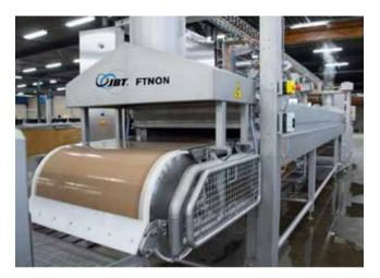
Steam tunnels with Teflon coated Kevlar belt:
