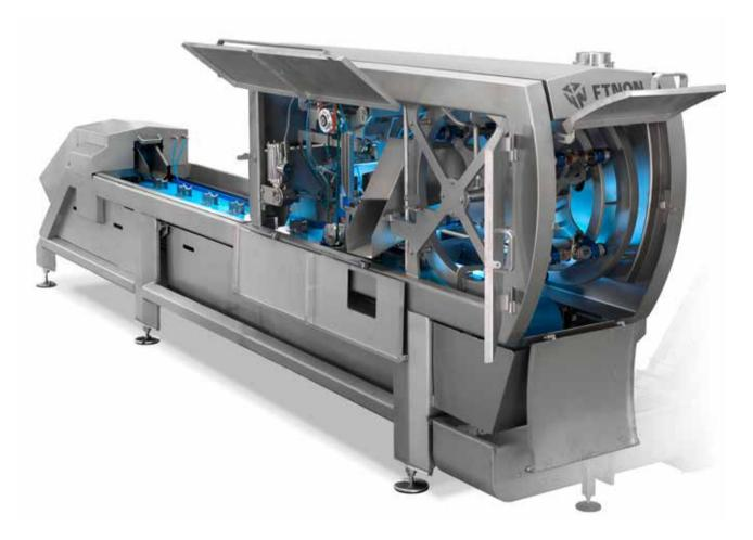
frictionless, based on magnetism, without springs, belts or other components. While rotating the onion around its own axes, another incision is made around the entire circumference of the onion. The incision depth can be regulated so that either one or more layers can be cut. A directed jet of air, limiting the air consumption, blows the cut skins from the onions. The waste is transported to a waste hopper via a funnel.
