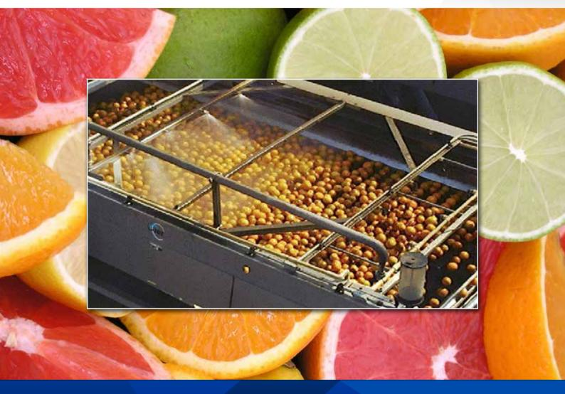
The JBT Brush Washer is designed to remove dirt and debris from the exterior of citrus fruit
