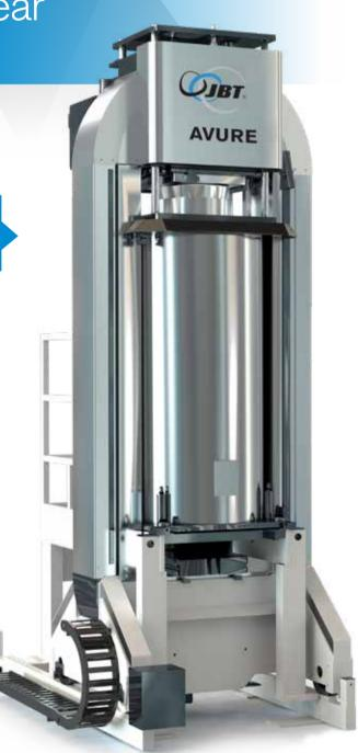
The AV-S is the only HPP system designed specifically for the seafood industry. Its vertical design increases yield in meat separation by up to 30% compared to other methods and prevents damage to the machine.
