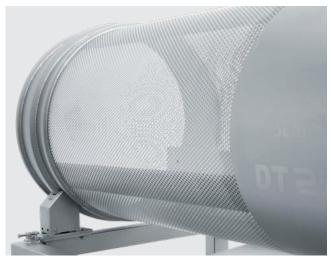
Perforated drum for brine drainage
