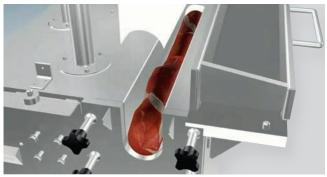
The meat is fed into the magazine using the sliding tray system
