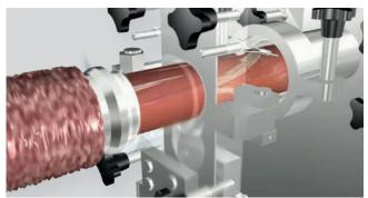
When the cutting unit is operating, the product in the HAMAX 800 is separated at the point it should be clipped
