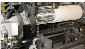
during the clipping process. The system is designed for the heaviest product weights. Designed to fit existing production flows, the looper is placed on the left side (second tie) of the machine.
