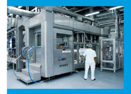
The JBT SF&DS AsepTec® is a reliable linear aseptic filler that stands out by the range of products and bottles (HDPE, PP, PET) it can handle at high line speeds. It was designed to provide carefully controlled and verifiable filling conditions.
