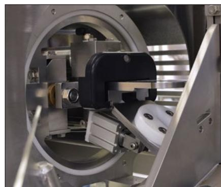
Optional handle maker consistently produces a correctly-sized loop with no wasted netting.
