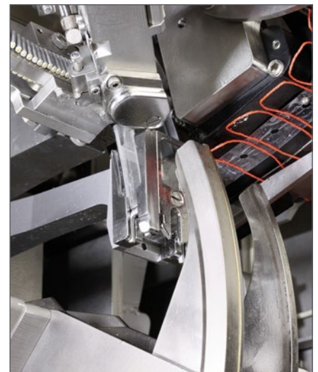
Shuttle clipping technology: voiding and clipping – precise, fast, consistent in caliber and gentle on the casing
