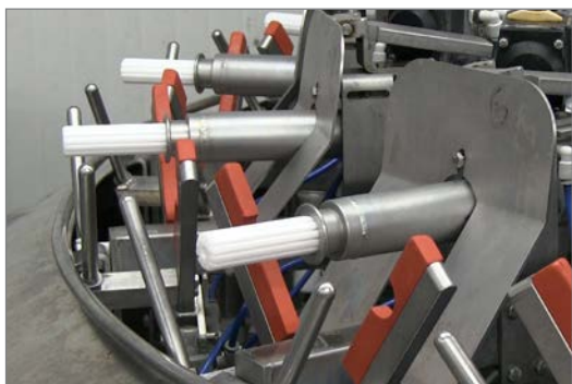
Fluted Teflon® probes ensure long-lasting performance.
