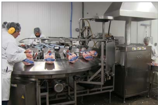
The Rota-Matic integrates easily with existing heat shrink systems for continuous, high-speed vacuum packaging.
