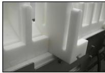
The TWS-1 Turkey Wing Segmenter is an innovative and safe solution designed to separate whole turkey wings into two or three pieces. Designed for either online or offline applications, this machine uses no rotating blades and delivers unmatched cut quality compared to other methods. The TWS-1 features Delrin products cavities for accurate loading, with quick-disconnect capabilities for trouble-free sanitation.
