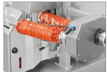
Two turret systems: V-turret head or parallel turret head for fast casing change.
