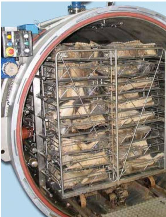
Trolley Handling by an Inner Trolley Chain
