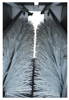
Pre-Scald Scrubber outfitted with stiff brush bristles removes fecal material and allows for quicker entry into scalder and reduces bacteria in the scalder.
