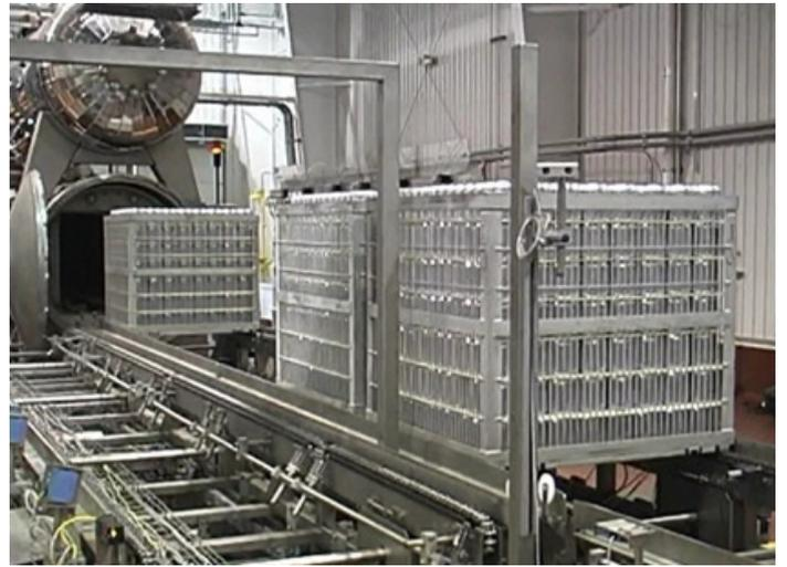
loader to pick up baskets for retorting. A fleet of conveyor-deck AGVs transports baskets from the loader conveyors to the batch retorts for high temperature cooking. Once the sterilization cycle is complete, the retort opens automatically and an AGV is sent for unloading. An AGV is ordered to remove the baskets and deliver them to the unloader or a buffer conveyor. AGVs also transport empty baskets to and from the buffer conveyors.
