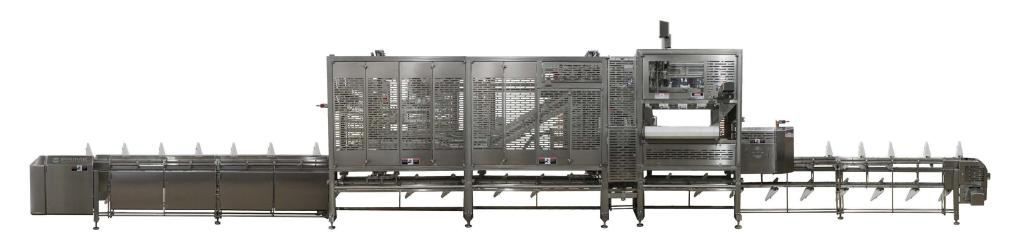
Prime's In-Line Breast Deboner for Turkey is an innovative approach to automating breast deboning that significantly reduces staffing, and provides consistent, high-yield results that meet or exceed cone line whole-muscle yields. With a small footprint compared to the cone line it replaces, the ILBD-2T is an efficient, labor-saving solution that solves multiple processing problems.
