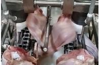
Breast cut from wings and dropped to conveyor
