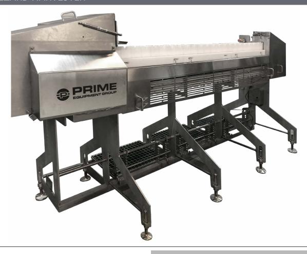
The GH-1T Gizzard Harvester from Prime Equipment Group is a high-capacity, efficient solution for separating heart and liver from turkey gizzards. Placed adjacent to the evisceration line and fed by evis workers as they remove internal organs, the GH-1T uses a rotary blade to slice between the heart/liver and the gizzard.
