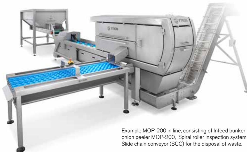
Example MOP-200 in line, consisting of Infeed bunker IFB-004, Magnetic onion peeler MOP-200, Spiral roller inspection system SRI-200 and a Slide chain conveyor (SCC) for the disposal of waste.
