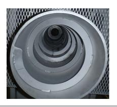
Prime DFS-Series De-Watering Screens are horizontally mounted, internally fed stainless steel wedge wire drums that effectively remove process water from various solid materials. Our most common separator applications are for skin and offal, but Prime also designs systems for other food industries. Various drum diameters are available up to 36 inches (91.5 cm) I.D., with lengths of up to 10 feet (304.8 cm).
