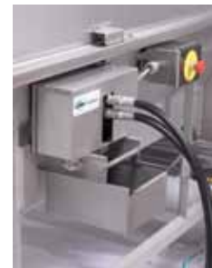
Crumb Box and Sifter Conveyor with E-Stop
