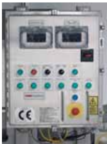
Control Box Hydraulic model: digital readouts for vertical screw, infeed discharge and drum speeds.
