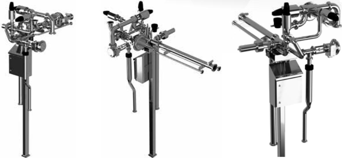
As an option for high volume machines (> 18.000 l/hr) the airbleeding valves can be replaced as well with a new type. This will increase the accuracy of the machine, especially during starting and stopping.
