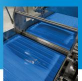
Machine redesign facilitates easy removal of the non-modular belt to make sanitation and maintenance more efficient
