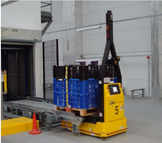
SGV drops off load at conveyor
