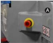
Red e-stop push buttons allow for immediate stops in case of emergencies.
