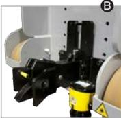
Optional automatic hitch reduces transition times between the AGV and cart to increase overall system productivity.
