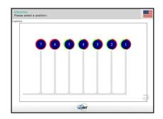
First swipe an ID card at the access terminal. Then, simply touch the position that corresponds with the location of the cart to be sent.
