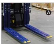
Single/double fork attachments support multiple load types and loading patterns.
