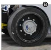
Soft, 18" diameter tires reduce wear on floors and improve traction.
