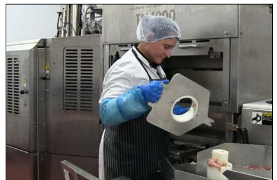
Easy tooling change without need for special tools.
